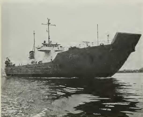
ARMY'S HIGH FLOATER—New shallow-draft amphibious resupply ship was developed through Army-Navy efforts.
